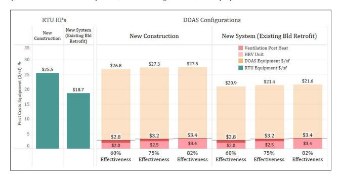
Figure 8: HRV/ERV first costs by each scenario evaluated compared with the total equipment costs for the DOAS system and compared with an RTU HP system cost (all other parameters include and averaged)
