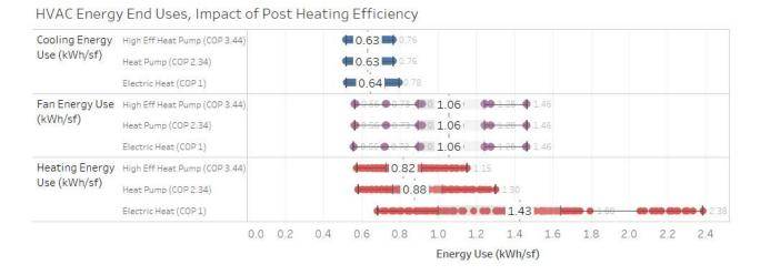
Post heating coil efficiency parameter, individual results of energy analysis averaged by end-use.
