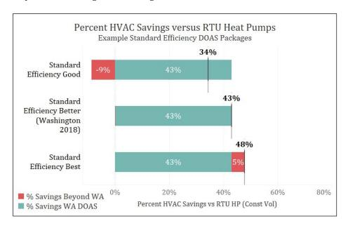
Figure 19: Percent HVAC savings versus RTU Heat Pumps for Standard Efficiency DOAS packages
