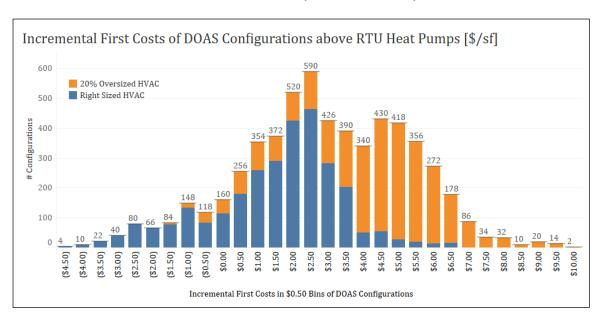
Figure 4: Incremental first costs of all DOAS configurations evaluated compared with the RTU HP baseline costs.
