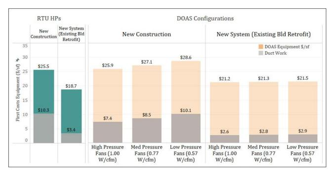
Figure 14: Ventilation HRV DOAS fan power parameter first costs by each scenario evaluated compared with the total equipment costs for the DOAS system and compared with an RTU HP system cost.
