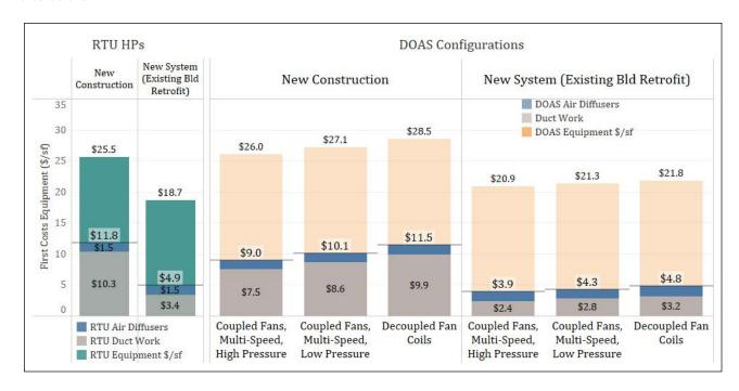
Figure 11: Coupled and decoupled ventilation configuration parameter evaluated compared with the total equipment costs for the DOAS system and compared with an RTU HP system cost.
