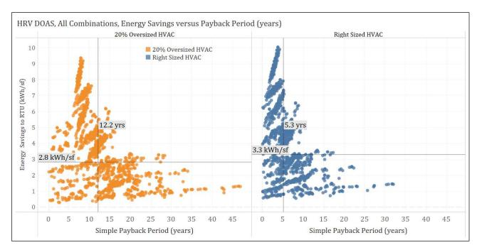
Figure 5: HVAC energy savings of each configuration versus RTU HPs by the payback period of the system in years. Information highlighted based on how cooling and heating systems are sized.
