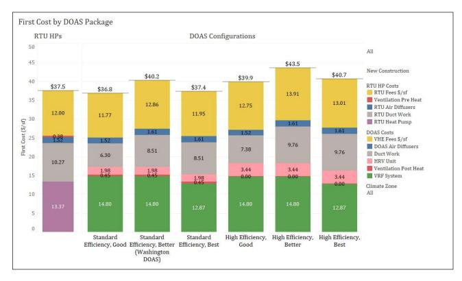
Figure 22: First Costs of Standard and High Efficiency DOAS example packages for new construction buildings
