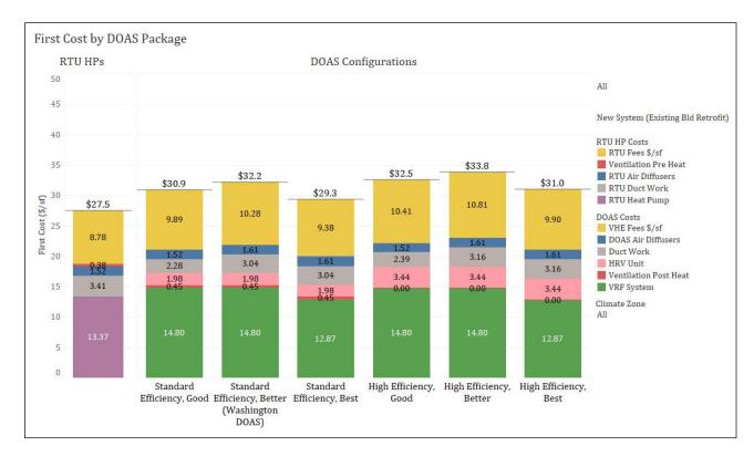
Figure 23: First Costs of Standard and High Efficiency DOAS example packages for existing buildings with new HVAC systems installed
