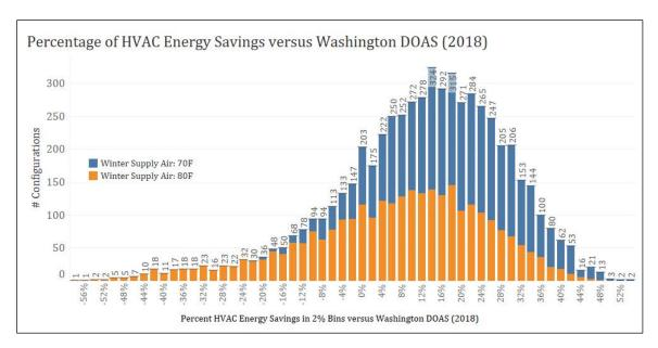
Figure 3: HVAC energy savings results for all combinations simulated compared with the Washington 2018 energy code DOAS configuration in bins of 2% energy savings by number of occurrences.
