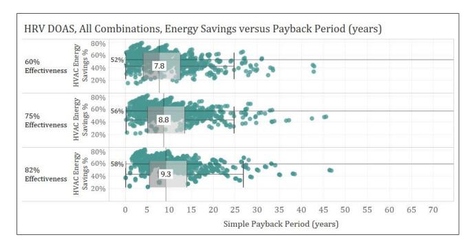
Figure 9: Simple payback period for HRV/ERV core effectiveness parameter evaluated compared with RTU HPs.
