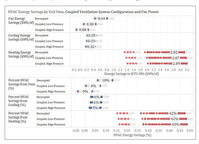
Figure 10: Coupled ventilation fan coils parameter, individual results of energy analysis averaged by end-use.
