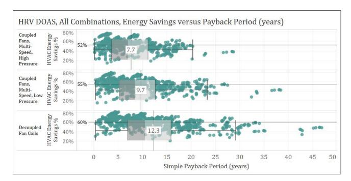
Figure 12: Simple payback period for Coupled and decoupled ventilation configuration parameter evaluated compared with RTU HPs.
