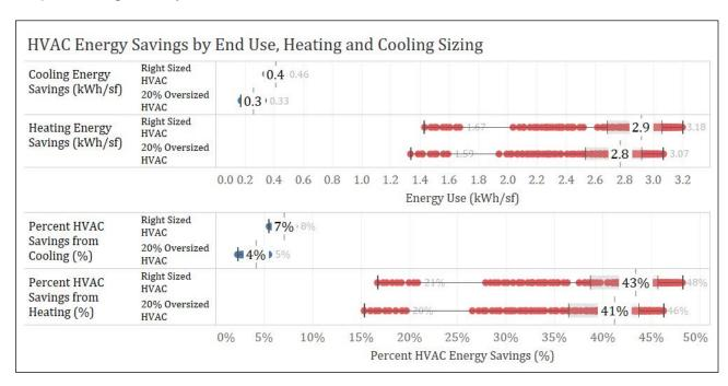
Figure 16: Heating and cooling system oversizing parameter individual energy savings for heating and cooling compared with RTU HPs.
