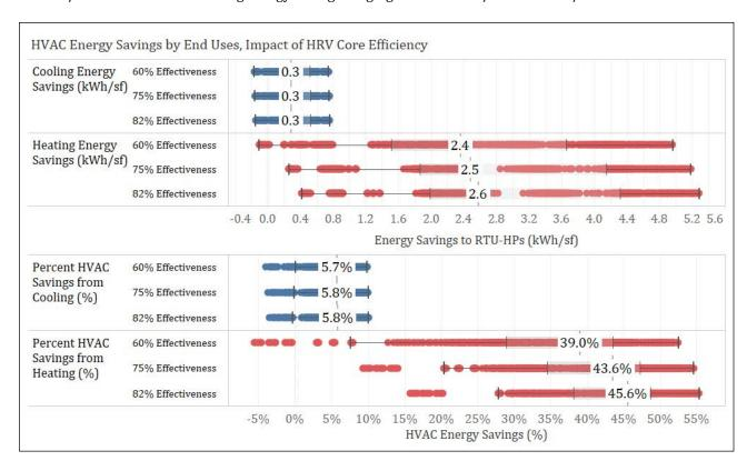
Figure 7: HRV core efficiency parameter individual energy savings for heating and cooling compared with RTU HPs.
