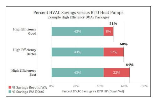
Figure 20: Percent HVAC savings versus RTU Heat Pumps for High Efficiency DOAS packages
