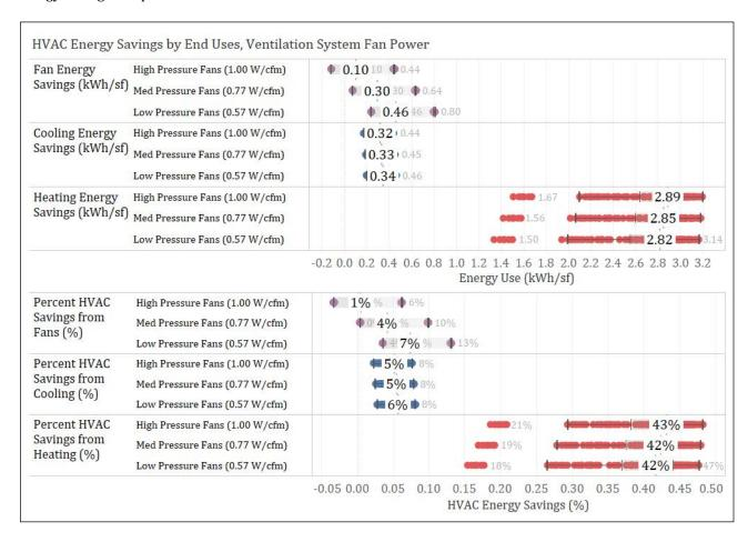
Figure 13: Ventilation HRV DOAS fan power parameter individual energy savings for fans, heating and cooling compared with RTU HPs.
