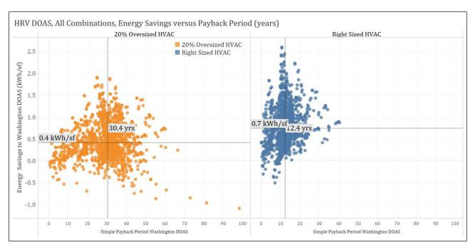
Figure 6: HVAC energy savings of each configuration versus the Washington 2018 energy code DOAS configuration by the payback period of the system in years. Information highlighted based on how cooling and heating systems are sized.
